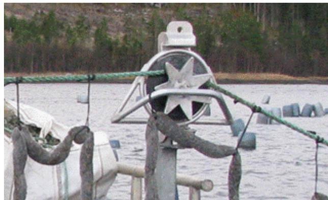
Figure 24 Mainline rolling through the starwheel
