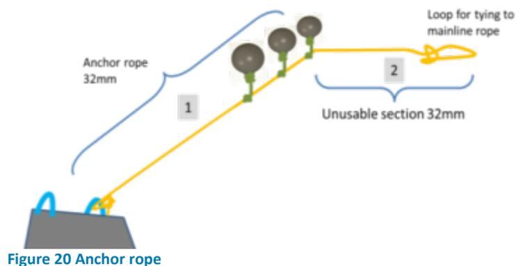
Figure 20 Anchor rope
