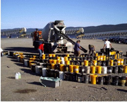
Figure 17 Production of compensation ballast weights
