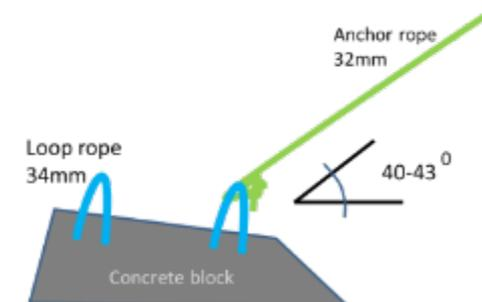
Figure 21 Anchor rope
