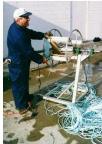
Figure 34 Rolling rope around spindle
