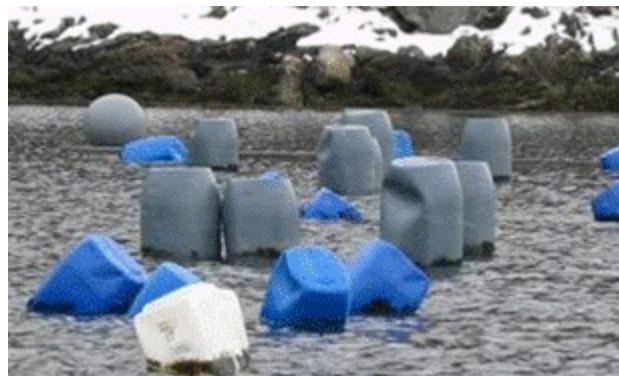
Figure 16 Inexpensive poor float quality
