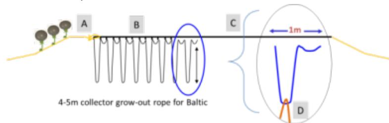
It may be advisable to test the addition of 2-3 kg armature bent into a V-shape on each long-loop of the collector during installation to make them sink if currents are strong to avoid collectors twisting.
