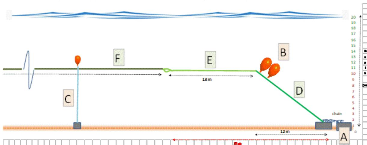
Figure 3 Schematic representation of submerged longline with primary components (A-F)
