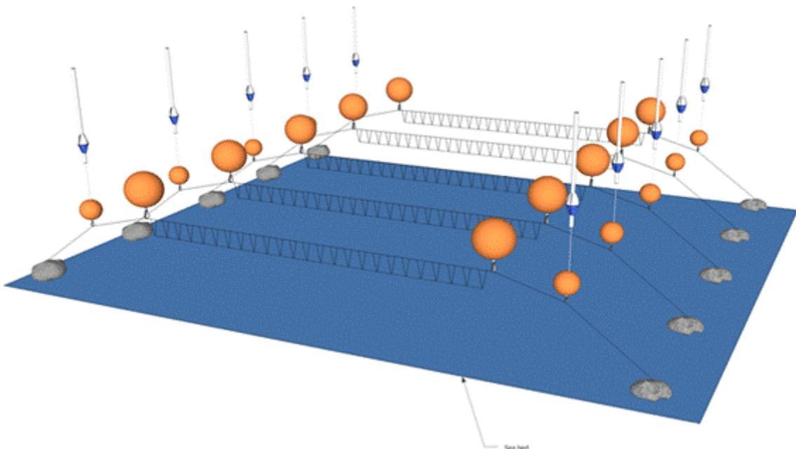
Figure 1 Overall design of the Latvian demonstration farm
